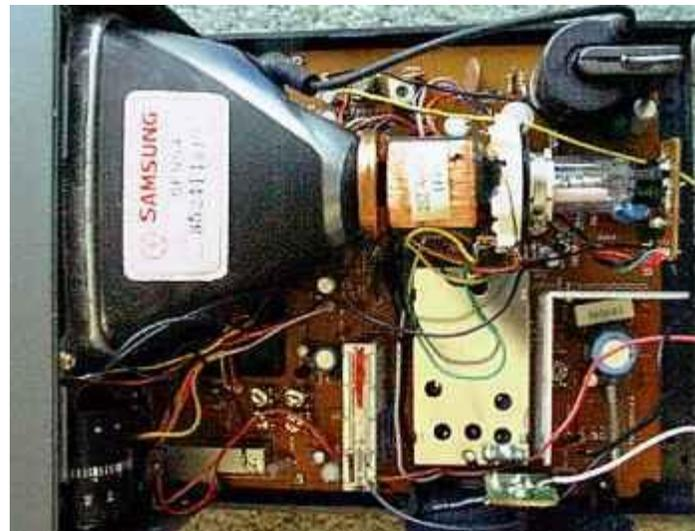
FIGURE 2 A TELEVISION SET WITH COVER REMOVED[4]
